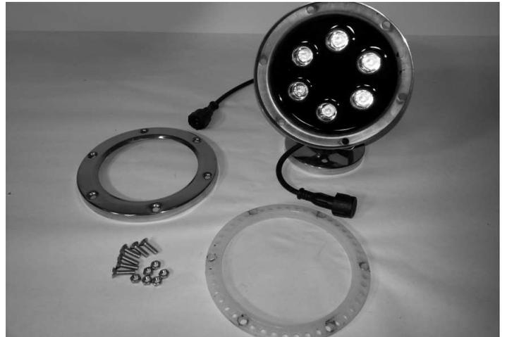
**MAINTENANCE:** Using an Alan wrench take off the screws and nuts. Remove the steel top ring. Take off the rubber ring and the glass. Clean any moisture or dirt. Replace the rubber ring and the glass cover. Make sure to align the holes in the rubber ring with the screw holes. Replace the top ring and install the screws
