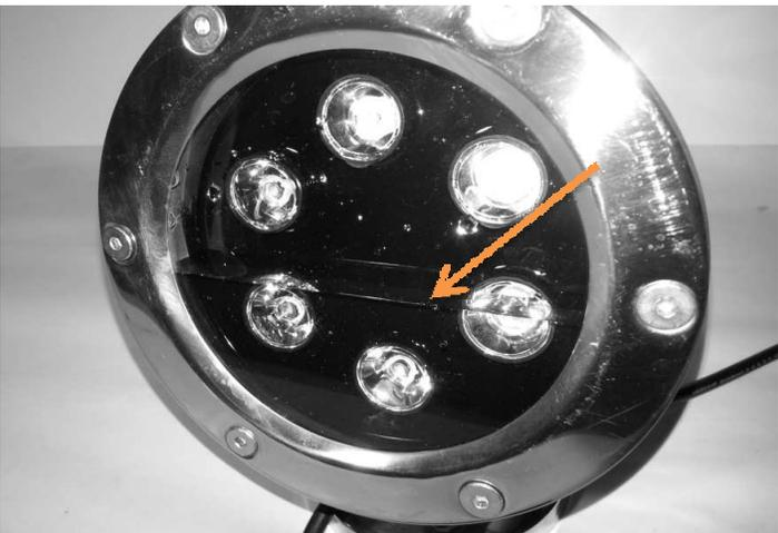
Presence of Moisture or water inside the glass is normal. The LED are sealed in resin and water or moisture will not cause any damage. Just perform maintenance periodically to get proper illumination through the LED and glass.
