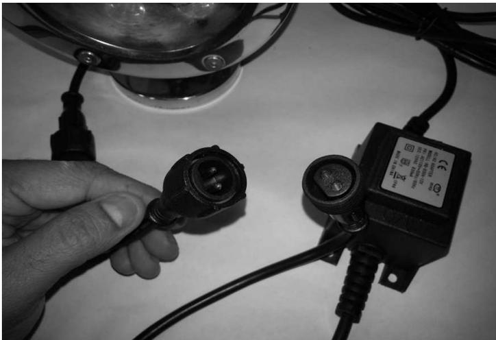
The Male connector of the LED Light gets connected to the Female connector of the ballast. This connection can only be complete one way due to the shape of each connector.
