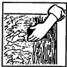
Removing damage with vertical straightline scratch pattern.
